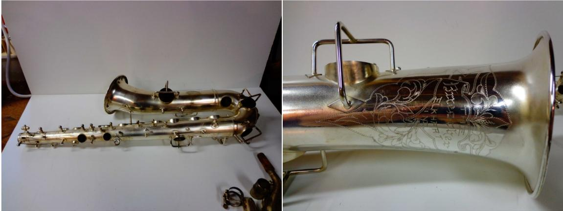
Next, the keys need attention. First job is to remove all the old pads. Depending on your preference, either an alcohol lamp or small torch works nicely. I use both, depending on how stubborn the pad might be glued and whether there is danger to parts or pearls on the pad cup.
