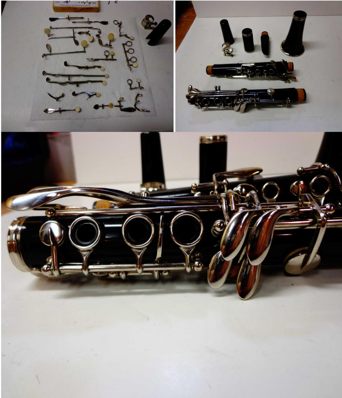
Fitting the correct size pad is very important, so I keep every size pad in stock in 1/2 mm increments so I can choose the best possible fit.
